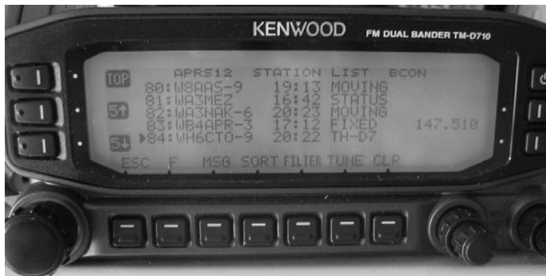
Figure 5. The new TM-D710 radio has a separate column for frequency in the station list. It also has a TUNE button to instantly QSY the radio to the indicated frequency.
