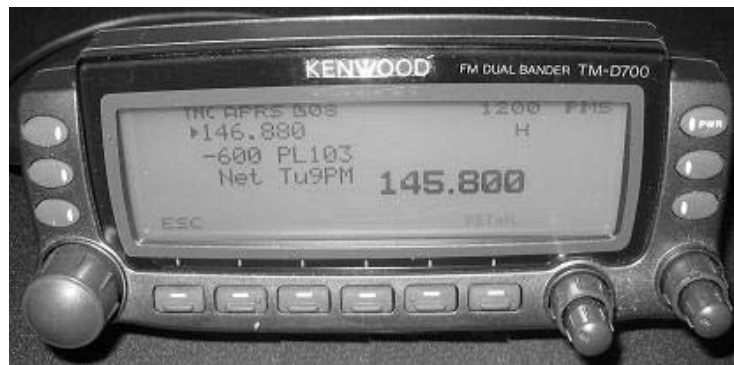
Figure 1. The local recommended voice repeater shows up on the left of the APRS screen. In this photo, I was using the right side of the radio to monitor for the ISS, when this local repeater object came in on the APRS channel.
