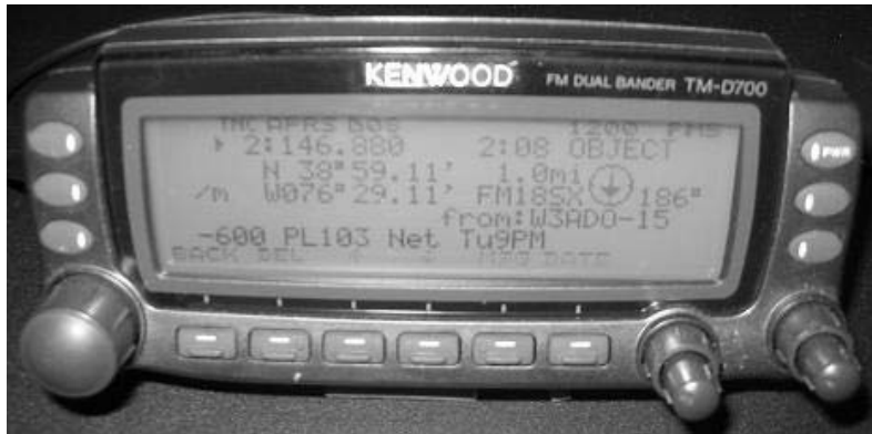
Figure 3. Once selected, the full details on this 146.88 repeater are shown. Again, the -600 and PL103 is no longer the final recommended format, being replaced with simply (-) in the frequency name and Tnnn for the Tone.
