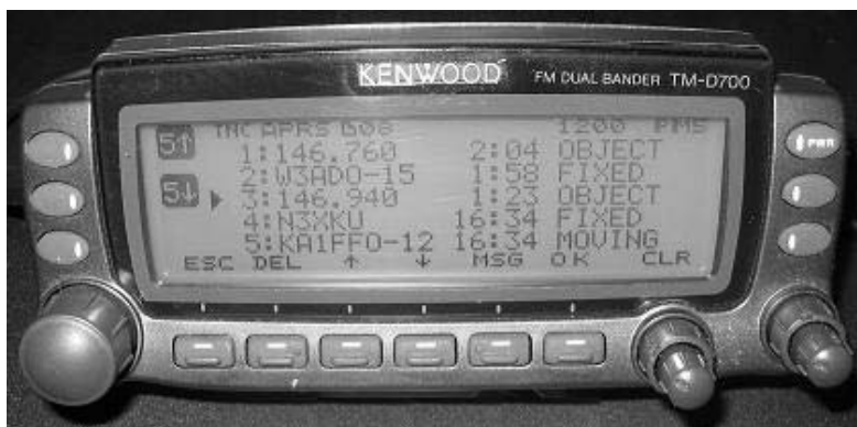
Figure 2. This photo shows how these Frequency objects show up in the station list for instant recognition.
