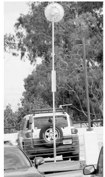
Figure 7 & 4 Examples of a Mid Mile node on a hitch-mounted multi-section flagpole
