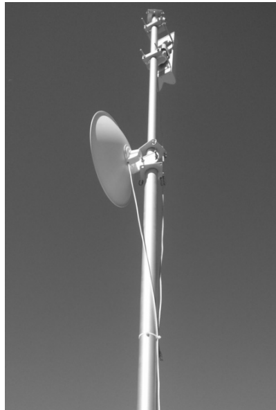
Figure 7 & 4 Examples of a Mid Mile node on a hitch-mounted multi-section flagpole
