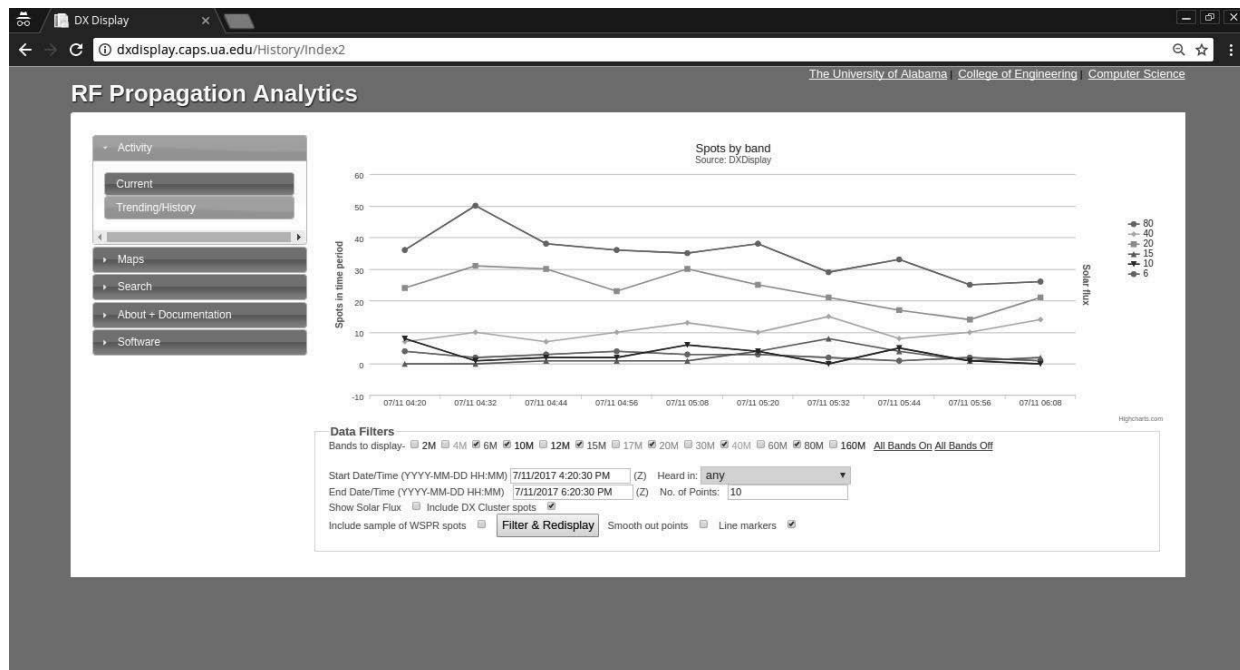
Figure 2: An automated propagation report system fed from multiple spotting networks. Built and run by William Engelke.
