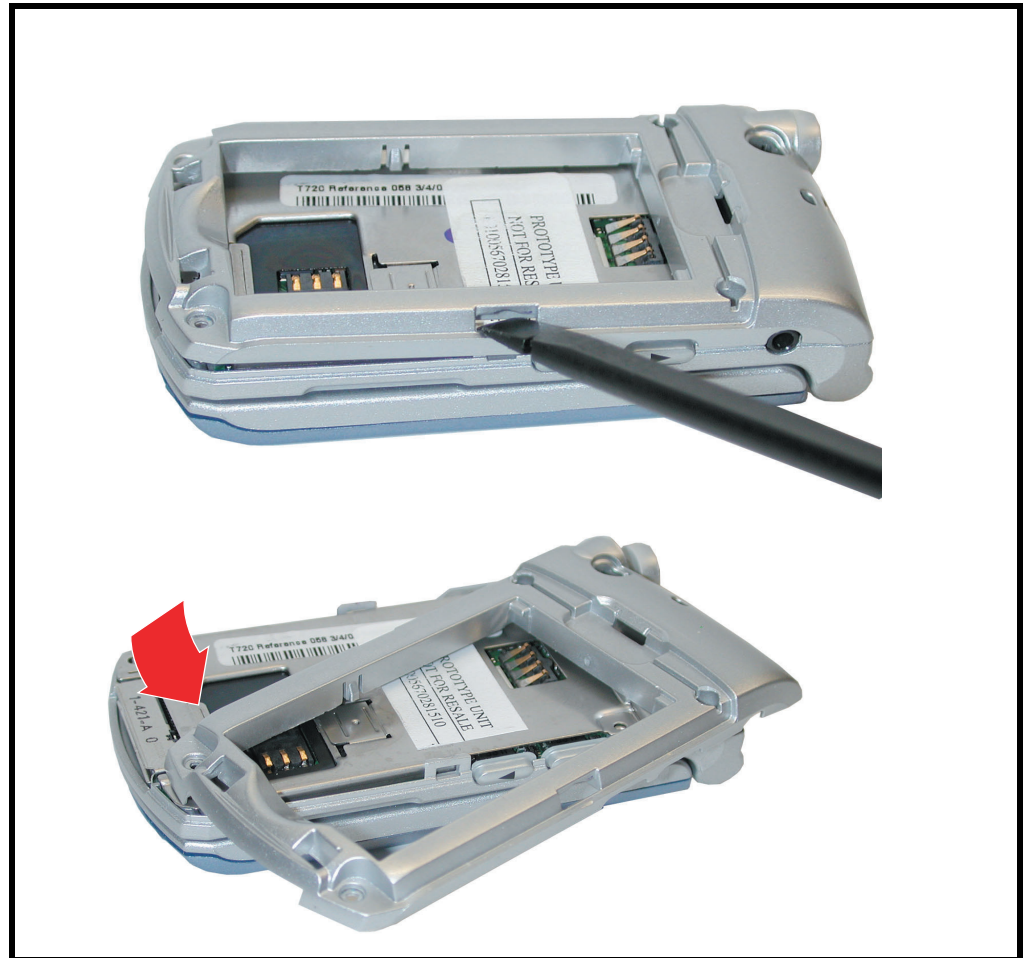
Figure 9. Removing the rear housing assembly
