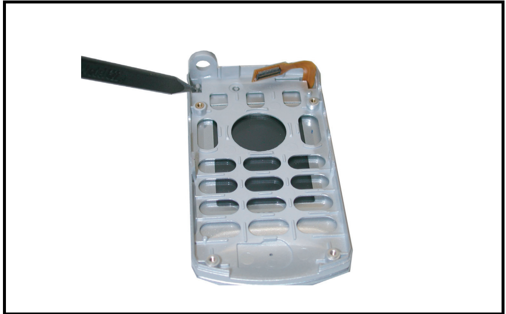
Figure 14. Removing the LED Light Guard
