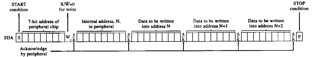
(a) General format to write to several peripheral internal registers or addresses.
