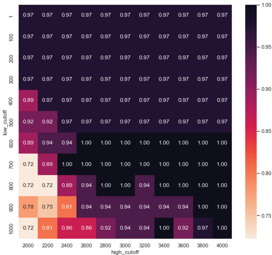
Figure 3. Heatmap for NATO phonetic alphabet recognition accuracy with various low and high cutoffs in Hz.
