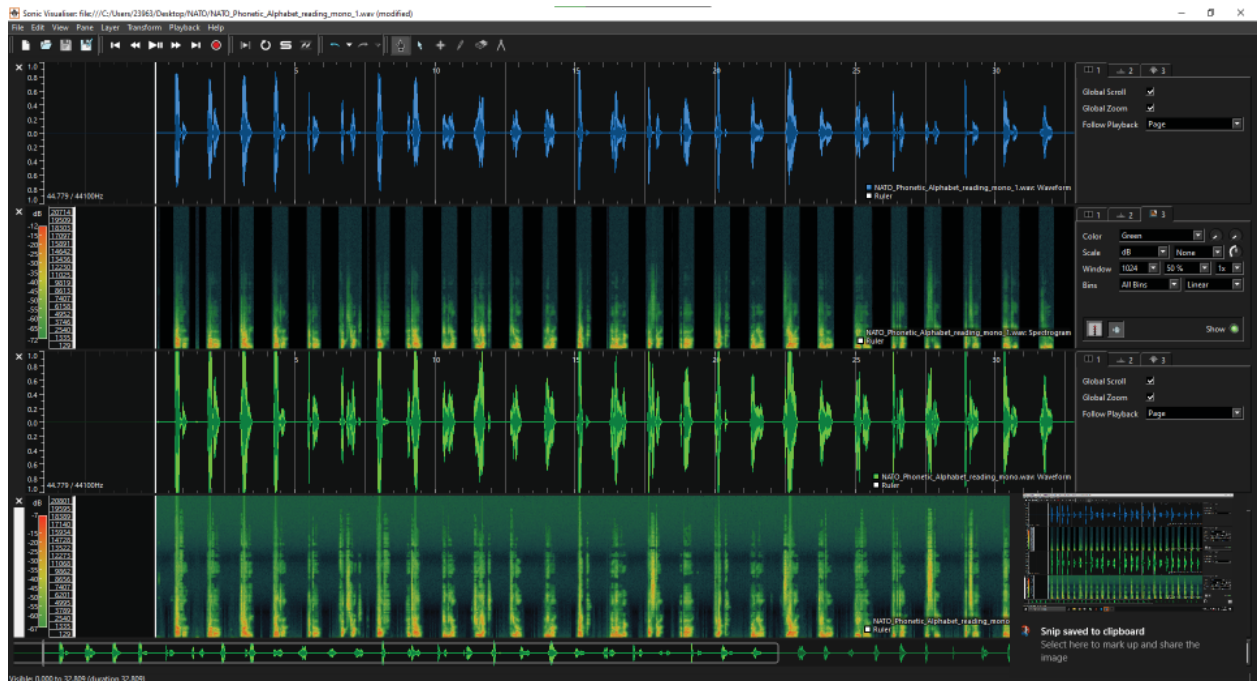
Figure 2. Visualization of the filtered spectrogram (top) vs. the original one (bottom). 300 Hz low cutoff and 2700 Hz high cutoff. Note the intensity difference at higher frequencies.
