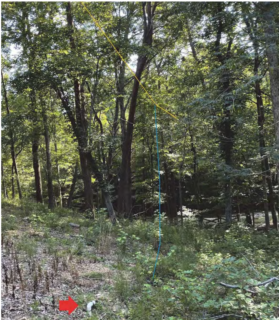
Figure 4. The 80M dipole is shown in false color to distinguish it from the trees; a red arrow points to magnetometer 2, installed in the worst possible location.
